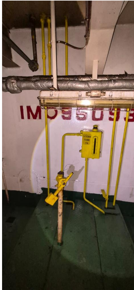
Image 29: Stern Tube Oil Seal Tank
